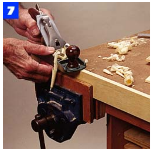
Clamp each rear frame piece in a vise and use a sharp hand plane to remove material down to the pencil line.
