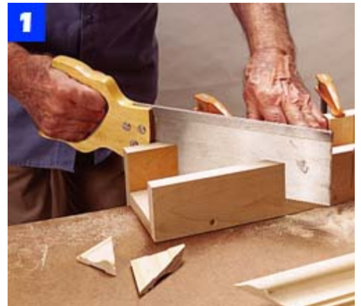
Cut the miters on the face frame. Use blocks to take up space behind the molding and to stop it from moving.
